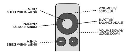
**Up and Down Buttons**: These normally function as Volume Up and Volume Down. In Menu mode, they function to move up and down in the menu as displayed on the operator display.
