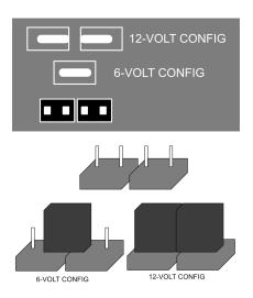
The MZ3 comes with selected old-stock 12SN7 tubes as its standard output tubes. By changing the jumpers on the circuit board, the amp can also use 6SN7 tubes. These are identical sonically, they simply use different voltages for the heater. When switching from one to the other, be sure to set the jumpers on the boards to the correct position. A 6-volt tube like the 6SN7 will burn out quickly if given 12 volts.
