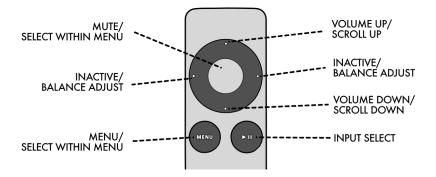
**Up and Down Buttons**: Volume Up and Volume Down. They can be held down or used in a single step mode. In Menu mode, they scroll up and down.
